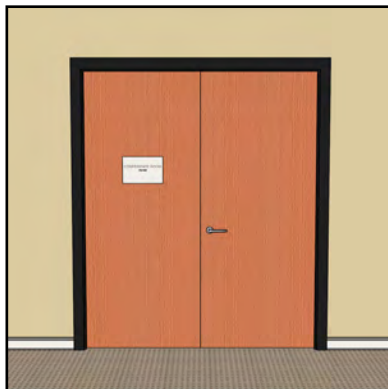
Sign on inactive leaf at double-door entry
