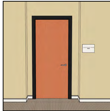
Recessed door with sign on adjacent wall
